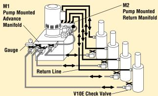
Many different system arrangements can be achieved by using a remote mounted directional valve. Remote valves are ideal when system control is desired away from the pump.
